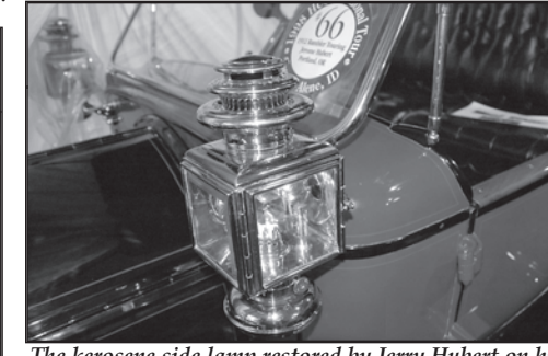
The kerosene side lamp restored by Jerry Hubert on his 1912 Rambler. Plated nickel that has been sprayed baked for maximum protection. A process Jerry has developed over 40 years ago.
