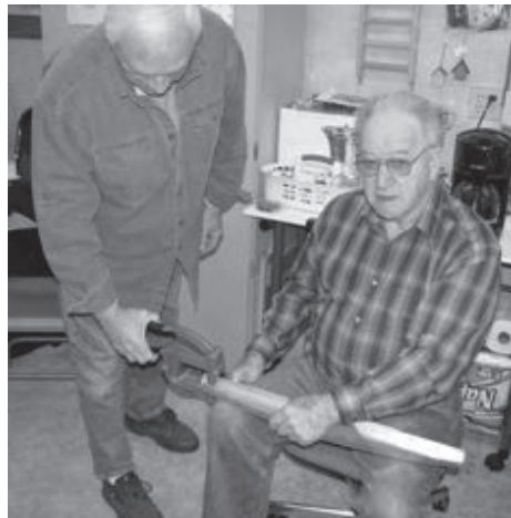
Russ Ashley demonstrates how Jimmie Fox's manual tool punches a hole through steel. It is available for club members to use.
