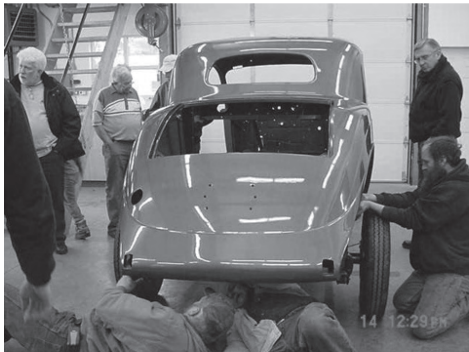
The work crew fastens the body to the chassis of Bill Marble's '35 Plymouth PJ Deluxe Business Coupe in his impressively equipped shop. Some of the visible participants were Tim McCarthy, Les Conner, Scott Farnsworth and Steve Marble.
