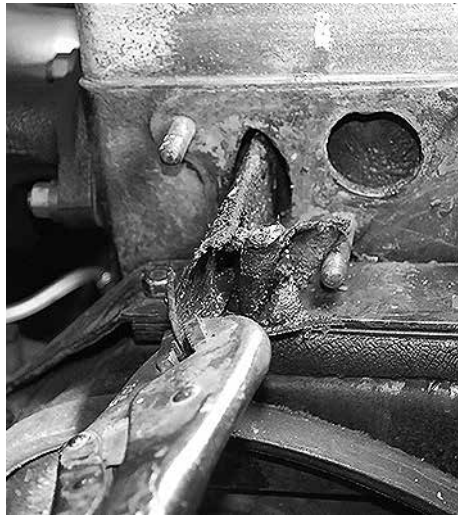
When you finally get hold of the water distribution tube, this is what it looks like. The grille needs to come out first.
