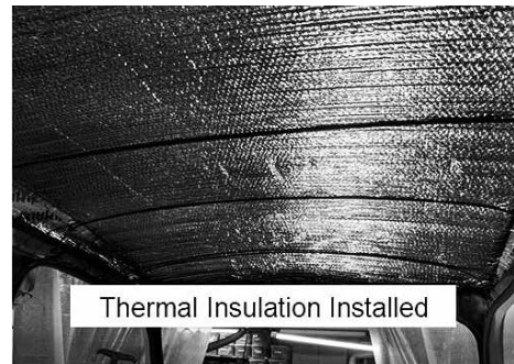
Sound Deadening Install
